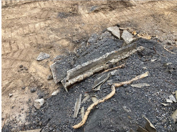
Examples of ACM in fill material
